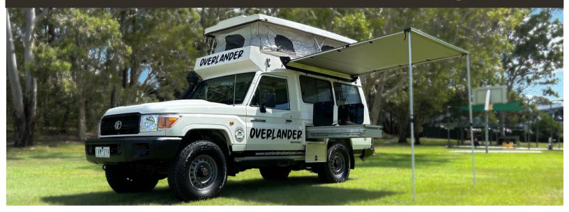
Toyota Landcruiser 4WD Camper is set-up for extended Long-Rang Touring with excellent off-road abilities and lots of space and seating for two. Equipped with slide-out kitchen with 2 gas burners and a sink, fresh water tank and upright fridge making it super easy to cook up a storm in even the most remote places. There are two beds for comfort and convienence.
